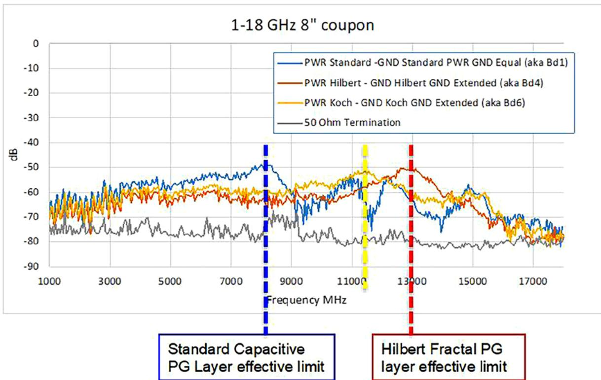
Figure 5: Changing small, unused features on a conductive layer can alter the PCB's electrical response.
