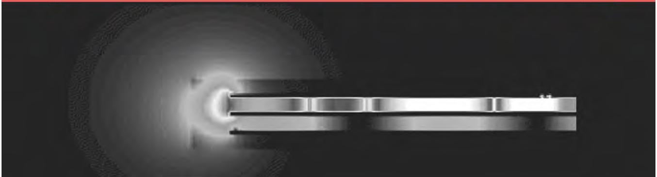
Figure 4: Description of the generating surfaces contributing to PCB edge noise.
