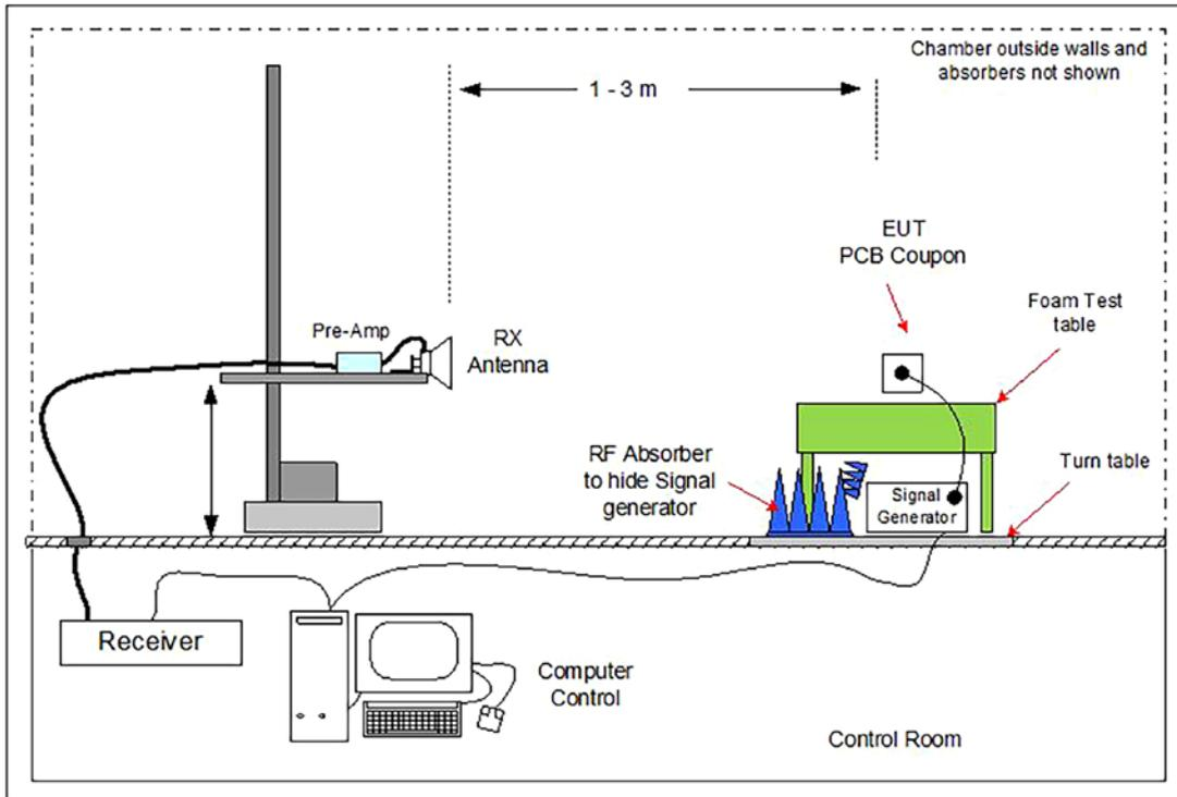
Figure 2: The test apparatus at a licensed FCC test and analysis laboratory.
