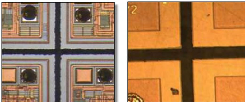
Figure 3: Comparison of a saw cut to a laser cut street-edge quality on a silicon wafer.
