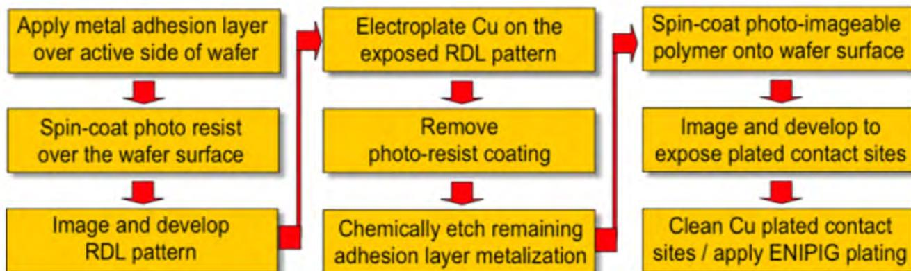
Figure 1: Basic RDL pattern imaging, plating, and etching process sequence.
