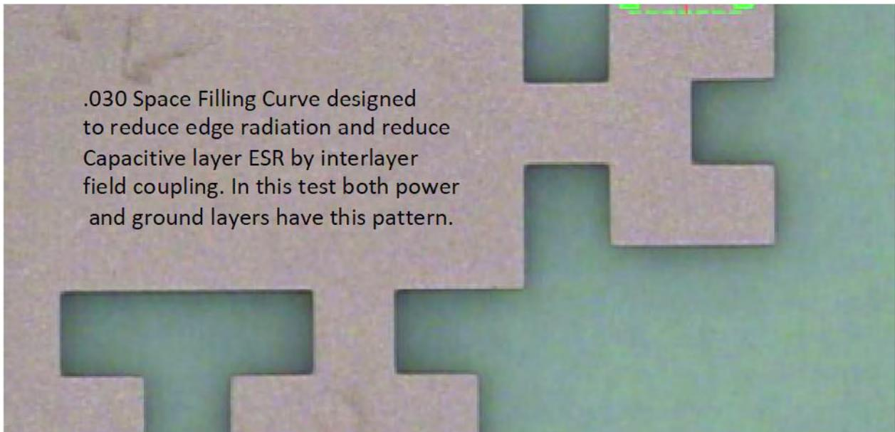
Figure 6: An experimental 0.030" proprietary Hilbert fractal edge pattern.
