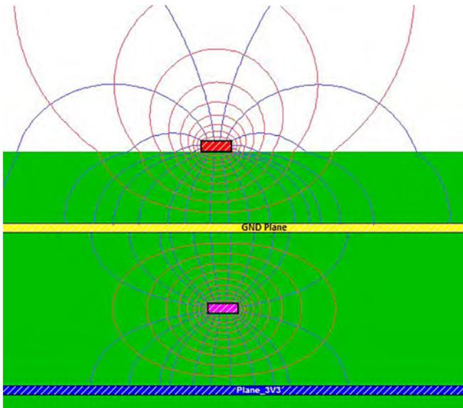
Figure 4: Microstrip and stripline electromagnetic fields. (Source: HyperLynx)
